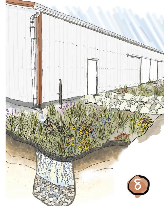
**Bioswales & Fish:** A bio-swale can be used in place of a traditional storm sewer. Planted with native, deep-rooted grasses, flowers, and shrubs, bio-swales beautify while holding and infiltrating water. Bio-swales work best when they are placed in existing drainage areas. By design, bio-swales infiltrate frequent smaller rain events and transport heavy rains without soil erosion. Bio-swales can be a good solution for areas that have problems with ponding and standing water.
